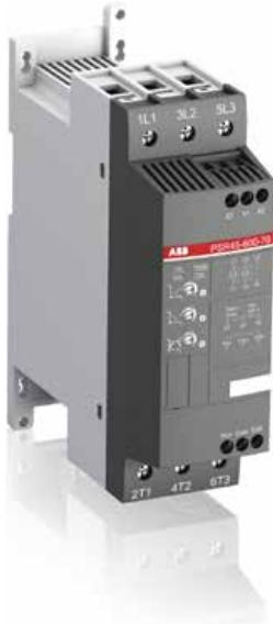
The PSR softstarter is the most compact of all the softstarter ranges which allows for design of compact starting equipment. A PSR together with a manual motor starter makes up a far more compact starting solution than a star-delta starter, and with the built-in bypass, the energy losses inside the softstarter are highly reduced.
